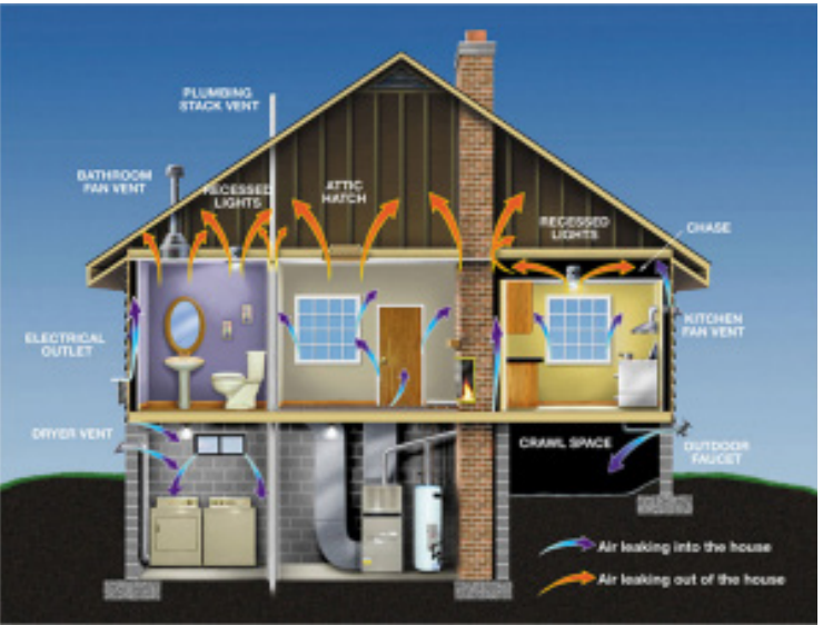
Above: Weatherization retrofits provide long term savings for low-income homeowners and renters. Measures can include air sealing, insulating walls or roofs, and improving ventilation, all aimed to reduce the homeowner's utility bills.
