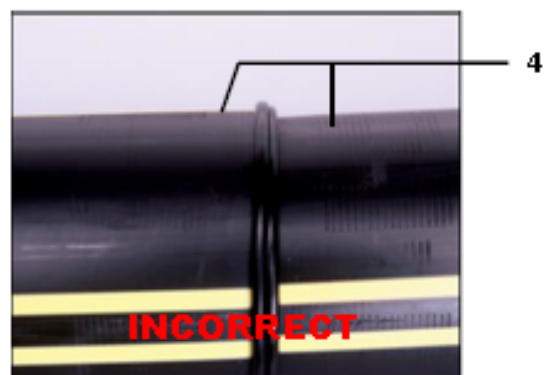
4. Improper "High-Low" alignment
