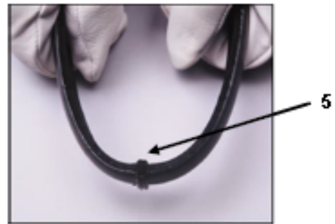
5. No gaps or voids when bent
